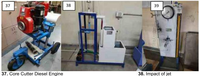
37. Core Cutter Diesel Engine
