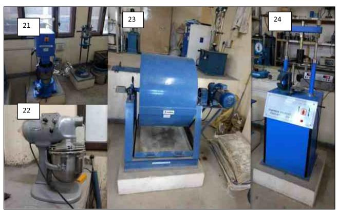
21. Bitumen Mixer/ Impact Testing Machine23. Los angles Abrasion testing machine
