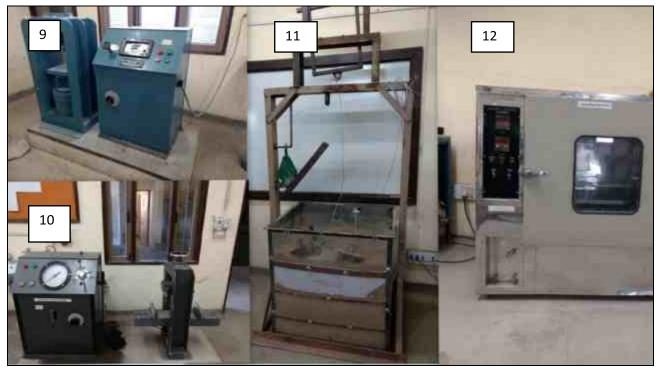
9. Compression Testing Machine11. Soil Pulling Apparatus
