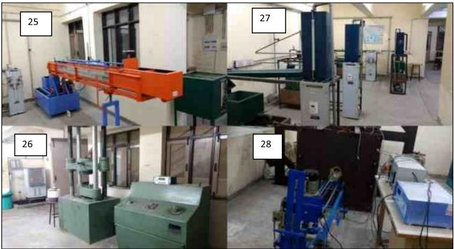
25. Open Channel Flume27. Apparatus for conducting orifice experiments (Cd, Cc, Cv)
